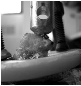
**Fig. 5.** Scaphoid model illustrating active compression producing displacement on the dorsal cortex between the proximal and distal aspects of the model.
