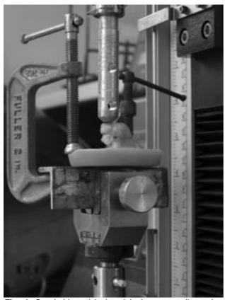
Fig. 4. Scaphoid model placed in Instron tensile testing machine to simulate compressive forces on the distal pole.
