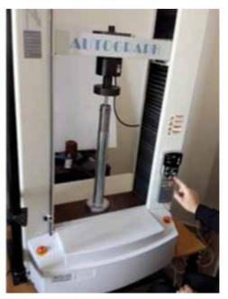
Figure 2. Illustration and photography of three-point bending test of locking screws.
