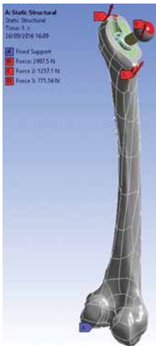
Figure 3. Prosthesis embedded femur model and load bearing conditions. Main force (applied to femoral head at 23° on frontal and 6° on sagittal planes) was taken to be 2997 N. Forces of abductor and iliopsoas muscles were taken as 1237 N (24° on frontal and 15° on sagittal planes) and 771 N (41° on frontal and 26° on sagittal planes).
